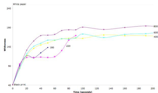
Figure 7: Print removed related to abrasive grit size (higher is finer), with 400g mass and at 200 rpm.
