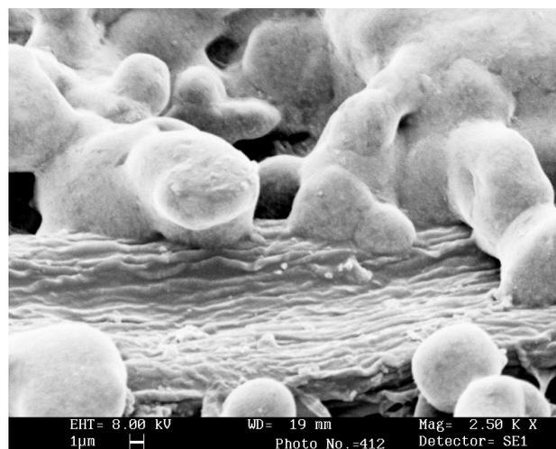
Figure 1: Electron microscope image of toner particles on cellulose fibre on surface of office paper (note that colour indicates electron transmission, not optical appearance).
