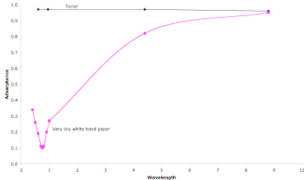
Figure 4: Absorptance of paper and toner adapted from Williams (1984) with wavelength measured in  $\mu\text{m}$ .
