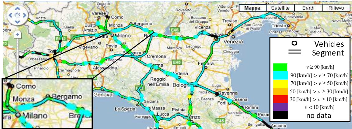
Fig. 1: Map of the North Italy motorways and look on A4 highway Milan→Brescia. Circles denote the vehicle velocities matched to highway segments.
